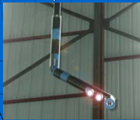
Tank Inspection Arm (Small Penetration, Low Payload)
