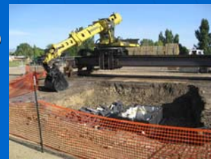
Graphite Reactor Decom. Arm (Very High Payload, Very High Shock, Long Reach)
