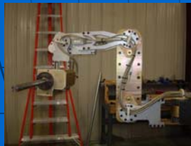
Reactor Inspection Arm (No Fluids, Advanced Controls)
