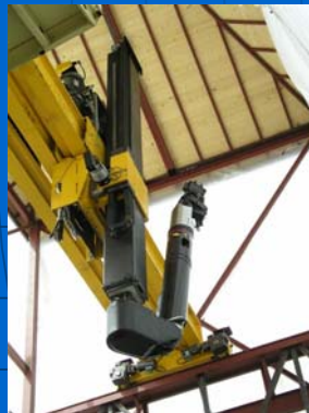
Graphite Reactor Decom. Arm (Very High Payload, Very High Shock, Long Reach)
