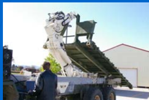
Pallet Loading Arm (Very High Payload, Moderate Controls)
